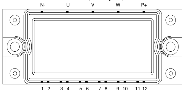
Pin out: APTGF20X60P2 (Short pins)
