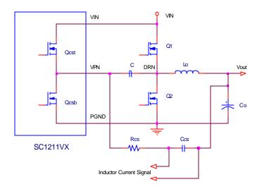
The above circuit shows the concept of Combi-Sense™ technique. An internal totem pole (Qcst, Qcsb) generates a VPN (Virtual Phase Node) signal. This VPN follows the DRN (or the Power Phase Node) with the same timing. A RC network (Rcs and Ccs) is connected between
