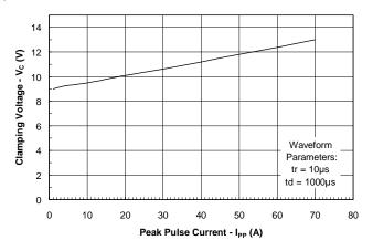
Clamping Voltage vs. Peak Pulse Current
