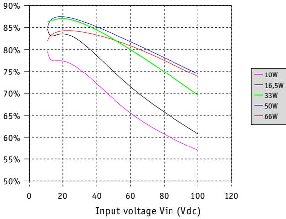
Fig 2 : Typical efficiency MGDS-100-M-C at 25°C
