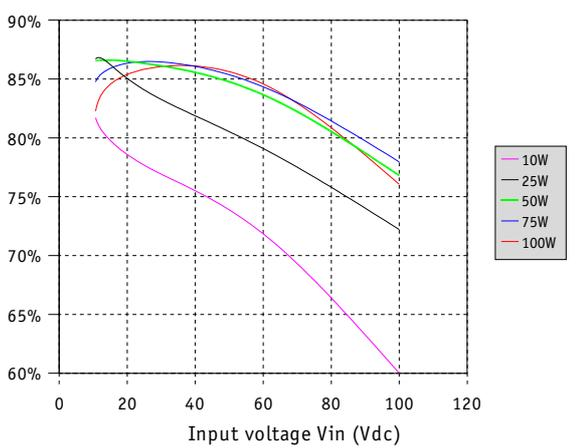
Fig 4 : Typical efficiency MGDS-100-M-F at 25°C
