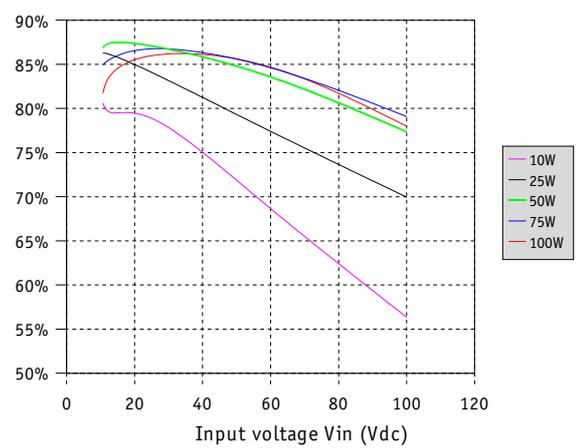
Fig 5 : Typical efficiency MGDS-100-M-26 at 25°C
