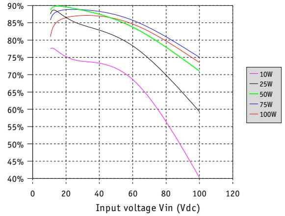
Fig 3 : Typical efficiency MGDS-100-M-E at 25°C
