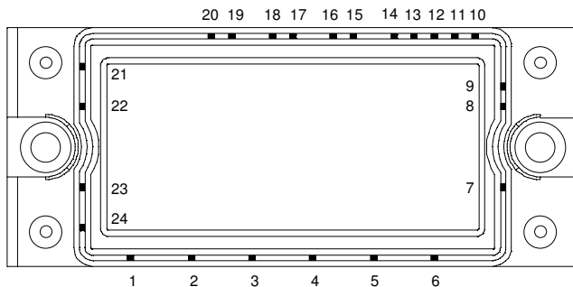
APTGS10X120RTP2: Without Brake (Pin 7 & 14 not connected)
