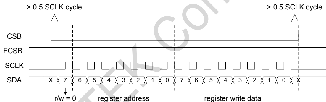
Figure 4-6. SPI write register timing
