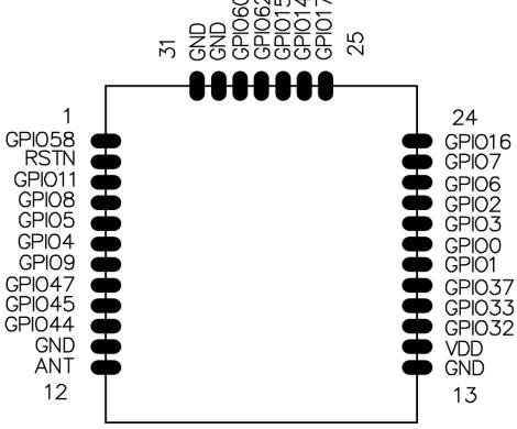
Figure 1. Pin Diagram Top View
